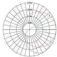
Maximum Candela = 2792 Located At Horizontal Angle = 0, Vertical Angle = 35
